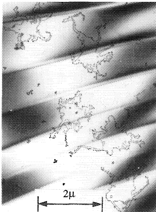
FIG. 3. TEM picture of monolayer etch pits on graphite basal plane. The sample was reacted in 21 Torr \text{H}_2\text{O} first at 730^\circ\text{C} for 2 h followed by \text{KNO}_3 deposition and further reaction at 700^\circ\text{C} for 3 h before gold decoration for TEM.
